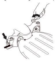
Rotate the blade and make sure you can still hold the rollers with your thumb when the blade is rotated.
