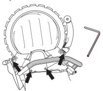
Rotate the blade and make sure that the support rollers are not clamped against the blade.
