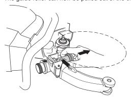
Screw the knob until it bottoms, and then loosen the knob 2 turns.
