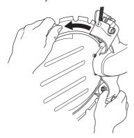
· Tighten the locking nuts on the support roller guard.
