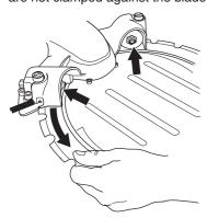
Adjust the adjuster screws so that the support rollers make contact against the blade.
