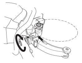
Insert the new guide roller in the chassis. Now press the guide roller into the knob.
