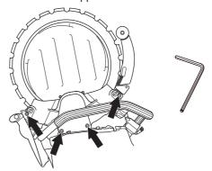
Use a 19 mm fixed spanner and a 13 mm combination spanner to replace the rollers.
