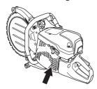
NOTICE! A dirty or blocked air intake results in the machine overheating which causes damage to the piston and cylinder.
