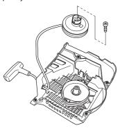
Bear in mind that the return spring lies tensioned in the starter housing. · Loosen the bolts holding the spring cassette.
