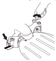
· Unscrew the adjuster screws a few turns.
